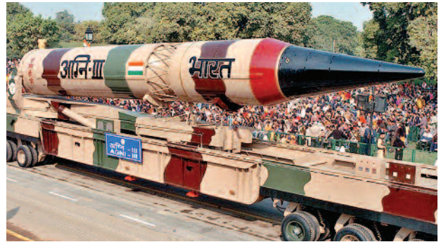
The Agni-III is an intermediate-range ballistic missile with a range of 3,000 – 3,500 km. It entered service with India's Strategic Forces Command in 2011, serving alongside the Agni-II as a nuclear delivery system.
